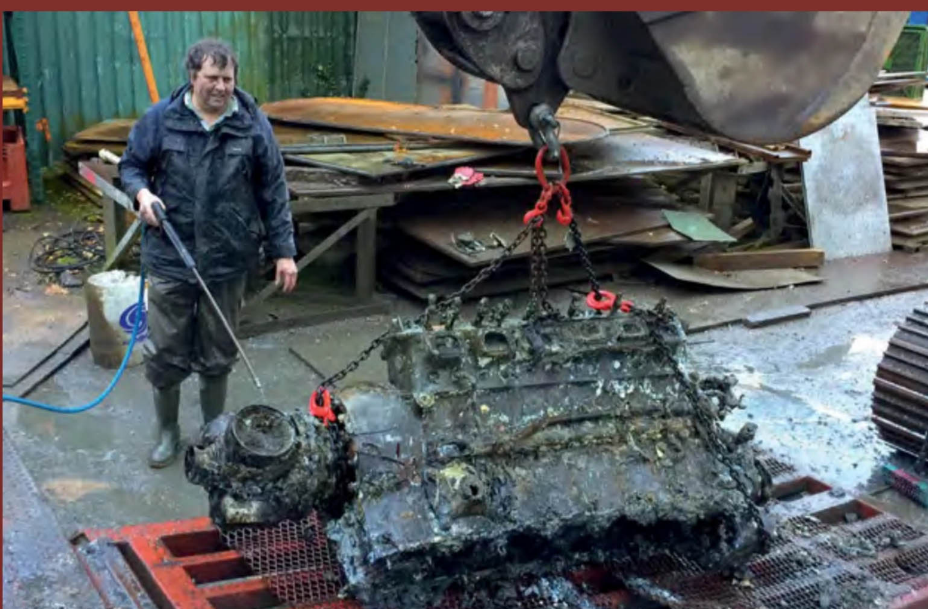
RIGHT Cleaning an engine from a dig is always a messy business and these needed further work to treat any remaining salt contamination, then many hours to remove the concretion adhering to numerous parts. (ANTONY ERIC WATKISS)
