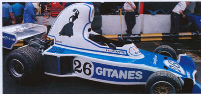
Bubbed the 'teapot', this gargantuan airbox appeared on the Ligier JS5 during the 1976 season
