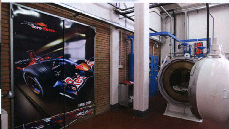
Above: the smallest of Toro Rosso's autoclaves. Bottom: team principal Franz Tost reflects on last year's win at Monza, his “greatest moment”
