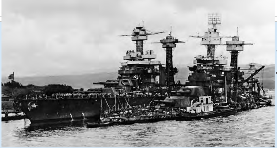
ABOVE: The battleship USS Tennessee is wedged against its mooring quays by the hull of the sunken USS West Virginia , which took several torpedo hits during the attack on Pearl Harbor. Engineers used dynamite to free the hull of the trapped Tennessee , which was repaired and modernized to later return to service. BELOW: The only capital ship of the U.S. Navy to get underway during the attack on Pearl Harbor, the battleship USS Nevada lies beached at Hospital Point and on fire after taking several bomb hits. The Nevada was repaired and returned to service, bombarding German shore installations during the D-Day landings in France. LEFT: A Japanese Aichi D3A Val dive bomber is seen in flight during the attack on Pearl Harbor. The Val is easily identified with its fixed landing gear. The aircraft was the frontline Japanese carrier-based dive bomber for much of World War II.
