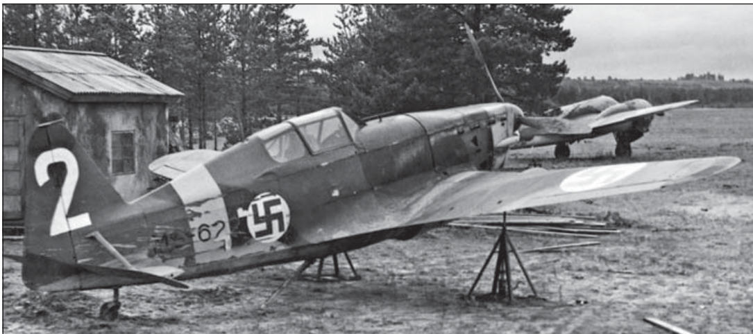
MS-622 of 2/LeLv 28 has been hoisted onto supports at Hirvas for undercarriage testing following a nose-up landing on 22 October 1942. The aircraft escaped without incurring any serious damage. It was regularly flown during this period by Sgt Pentti Piispa ( Finnish Air Force )
