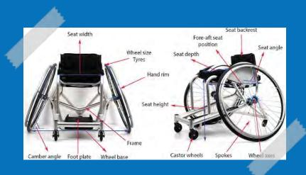
Most of us don't realise that there are multiple possibilities to adjust the configuration of a tennis wheelchair. The wheels and castor wheels directly influence the interaction between the wheelchair and the court surface.
