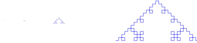
Fig. 5.2: Koch curve generated by the L-system F \rightarrow F + F - F - F + F after 0, 1, 2 and 3 expansions.
