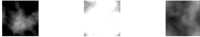
Fig. 4.3: Three hight maps generated the diamond-square method. The parameters used are: iteration = 9 for all maps, seed = 12, 128, 128 and roughness = 256, 256, 128 for the first, second and third map, respectively.
