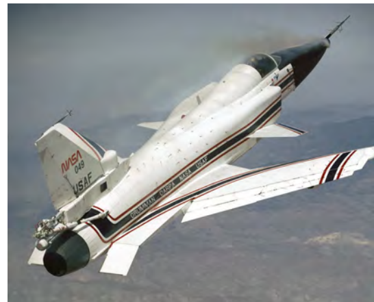
The second X-29 (complete with anti-spin 'chute fairing on the tail) conducts high angle of attack testing with smoke generators NASA
