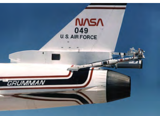
An in-flight close-up of the anti-spin 'chute fanning on the tail of the second X-29 NASA
