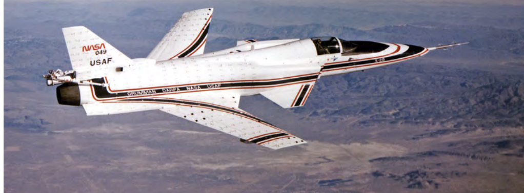
In this image a number of 'tufts' have been placed on the wings and fuselage of the second X-29 to allow high definition cameras to analyse the airflow across the airframe at high angles of attack NASA - Larry Sammons
