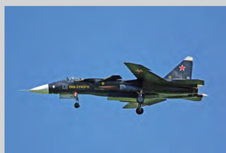
Seen landing back at Zhukovsky during an early test flight the Su-47 demonstrates the undercarriage it shares with the Flanker family of Sukhoi jets Viktor Drushlyakov
