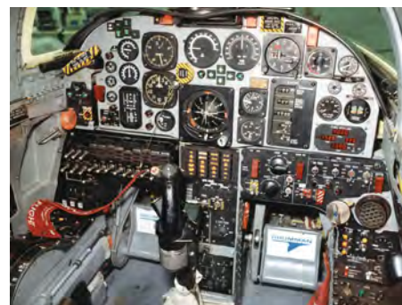
The X-29 cockpit borrowed much from the Northrop F-5 Freedom Fighter from which it was developed NASA
