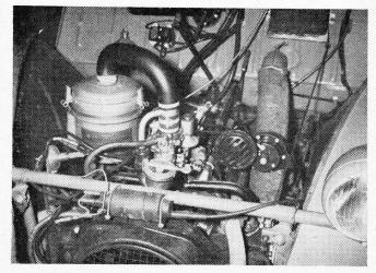
FRONT engine (above) is normally fitted and drives the front wheels only as in the existing 2CV.
