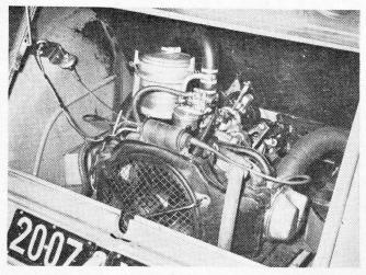
REAR engine (above) drives the back wheels only, and can be started or stopped independently of the other.
