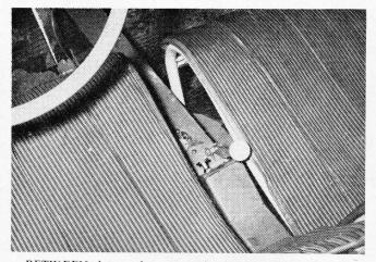
BETWEEN the two hammock-type front seats is the starter control for the rear engine.
