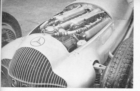
ENGINEERING MASTERPIECE: The superb and complex power-unit of the 1938 Mercedes-Benz. As with Auto-Unions, these cars were state-subsidized. The enormous cost of these cars would make this type of racing prohibitive these days.
