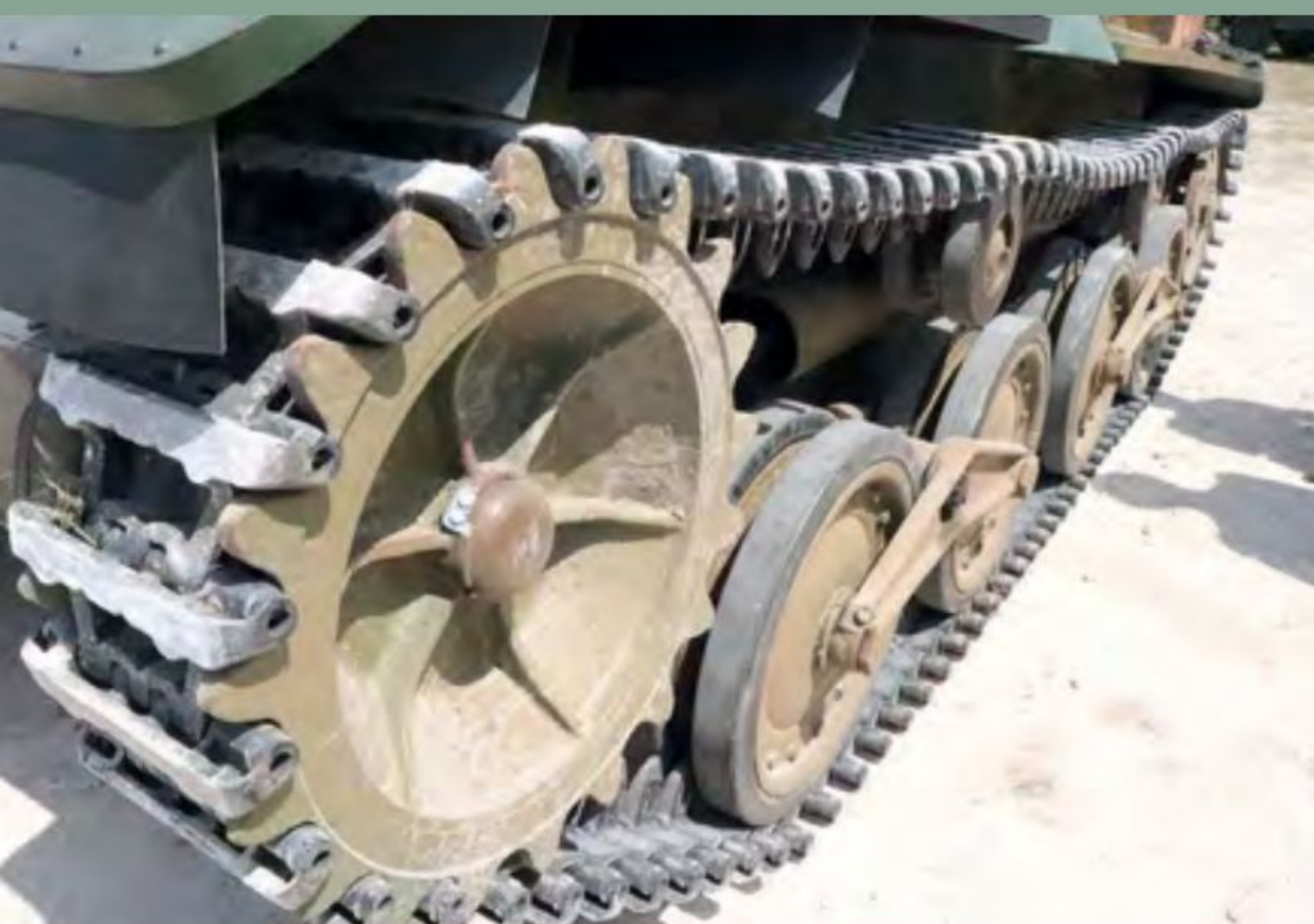
The tracks were driven through the front sprockets. ANDREW STONE
