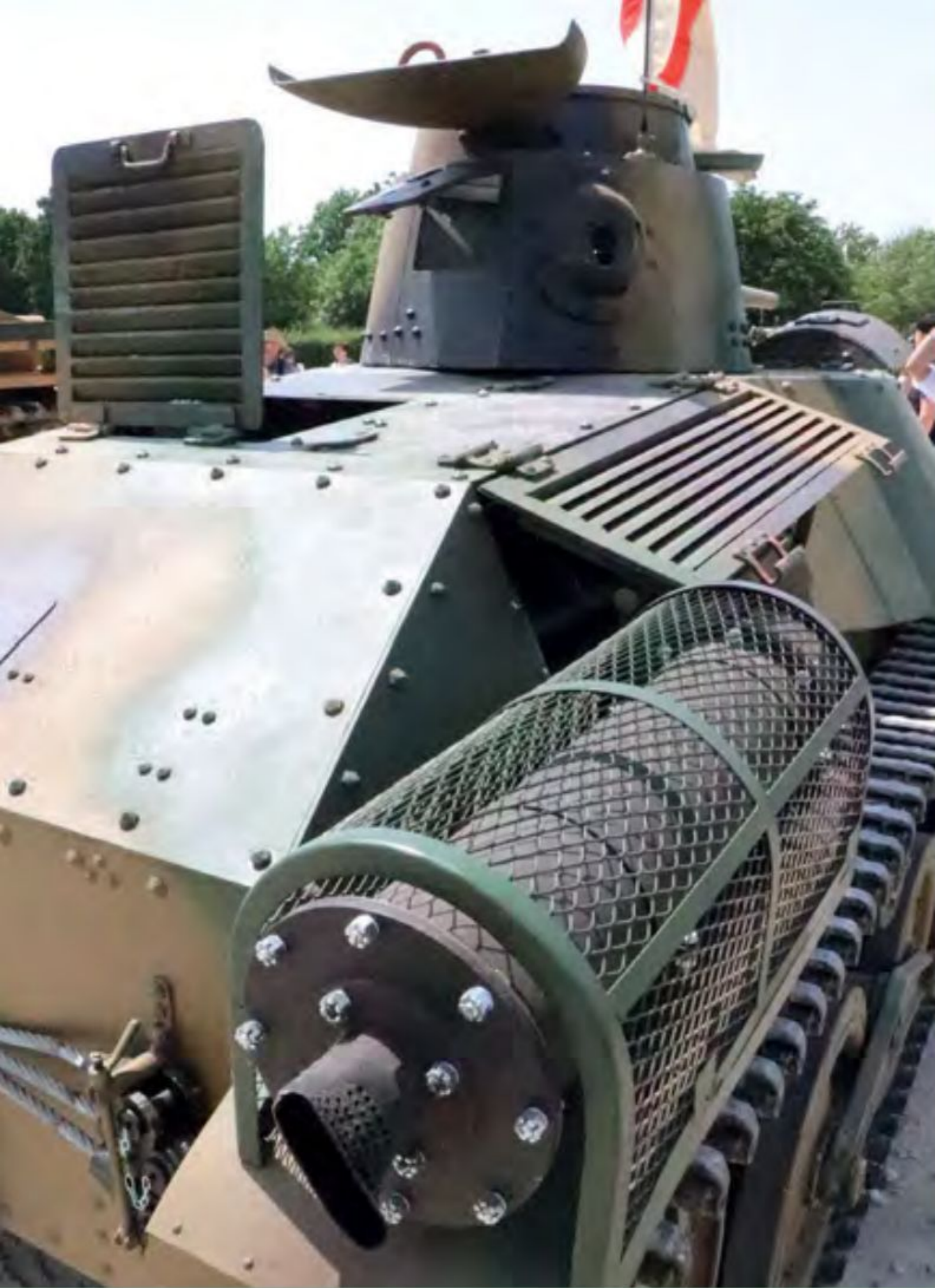
A view from the rear of the exhaust with protective cage. ANDREW STONE
