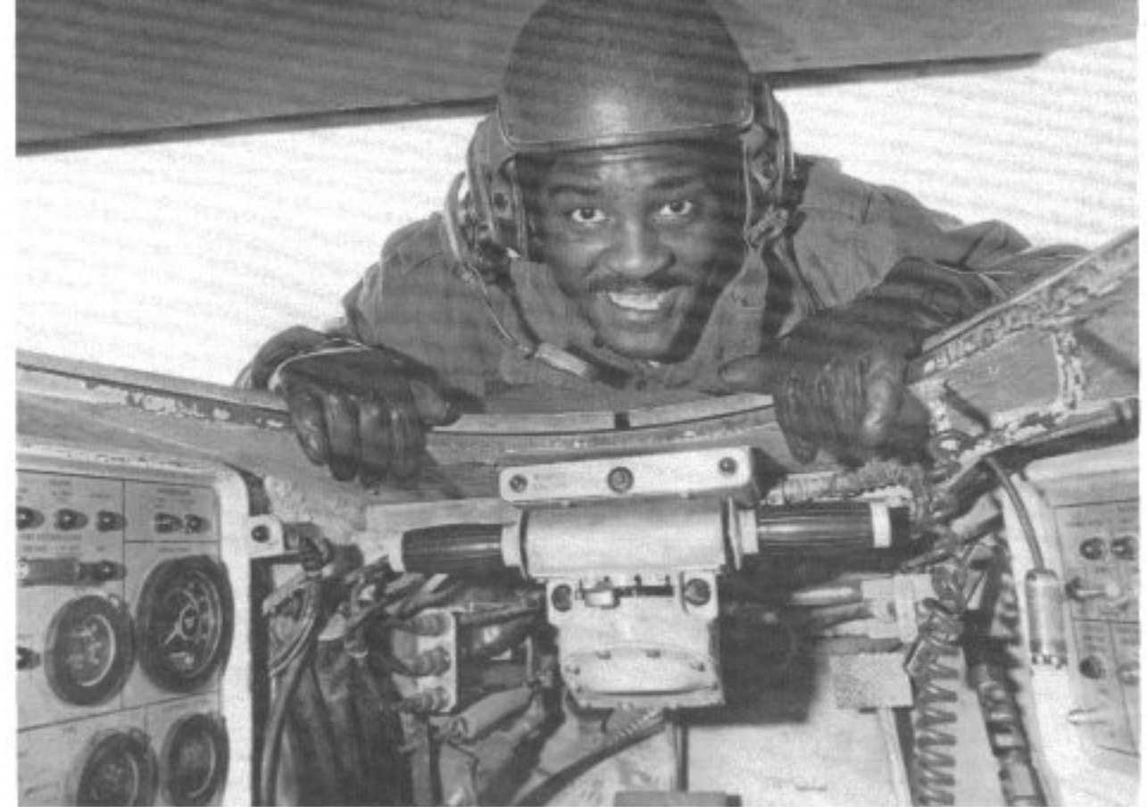
The M1's driver sits in a reclining position in the front center of the hull surrounded by his controls. The main driving controls are a set of motorcycle type handlebars which can be positioned in a number of ways depending on the wishes of the driver. (U.S. Army via Wagner)
