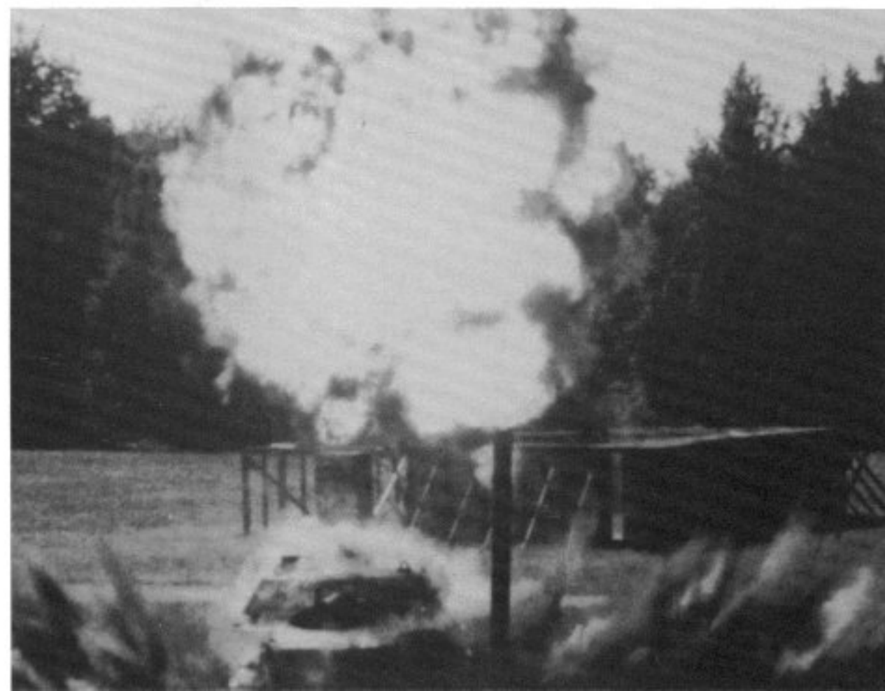
One of the most spectacular survivability tests was the explosion of an artillery shell directly over an M1 to test the thinner top armor. The shell was detonated above the turret electronically to determine how an airburst would affect the tank. (Green)
