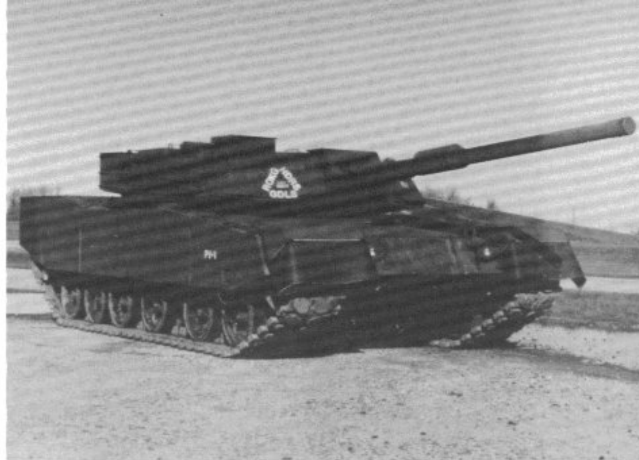
The similarity between the M1 and the South Korean XK-1 is not accidental because the contractor, Chrysler/General Dynamics used much of the experience gained with the M1 project in its design. The XK-1, however, has a lower profile and is some eight tons lighter than the M1. (Green)
