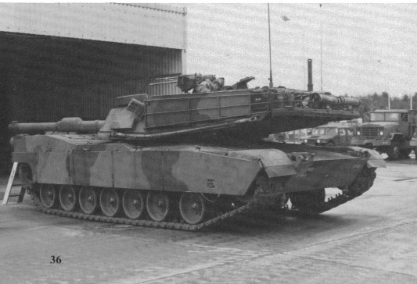
Production M1A1s began arriving in Europe during the Summer of 1986 carrying a new three tone Forest Green, Red Brown, and Black camouflage scheme in a special chemical resistant paint. (Jerchel)
