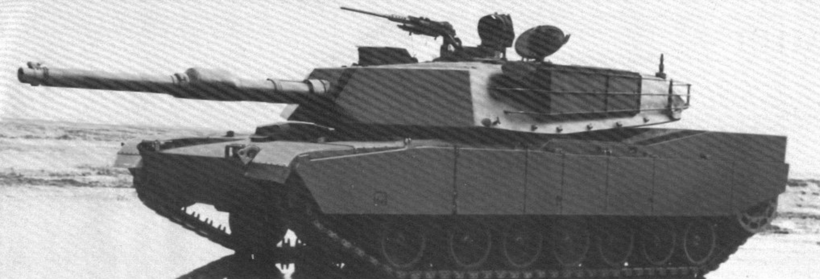
This early M1E1 lacks the simulated armor weights and stowage rack on the rear of the turret. The turret stowage boxes were later modified to extend all the way to the rear of the turret. (U.S. Army)
