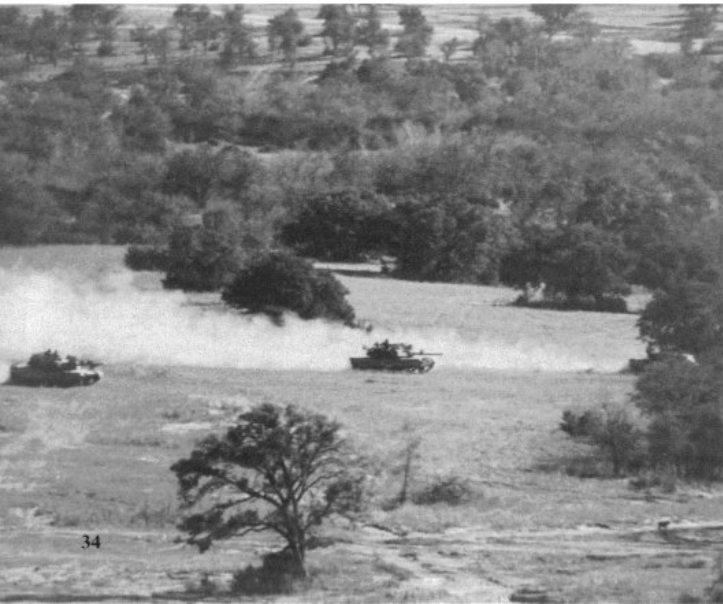
(Below) M1s moving cross country at high speeds can create a large dust cloud. The M1 can also create a deliberate smoke screen by using its grenade launchers and engine smoke generator when under enemy fire. (U.S. Army)
