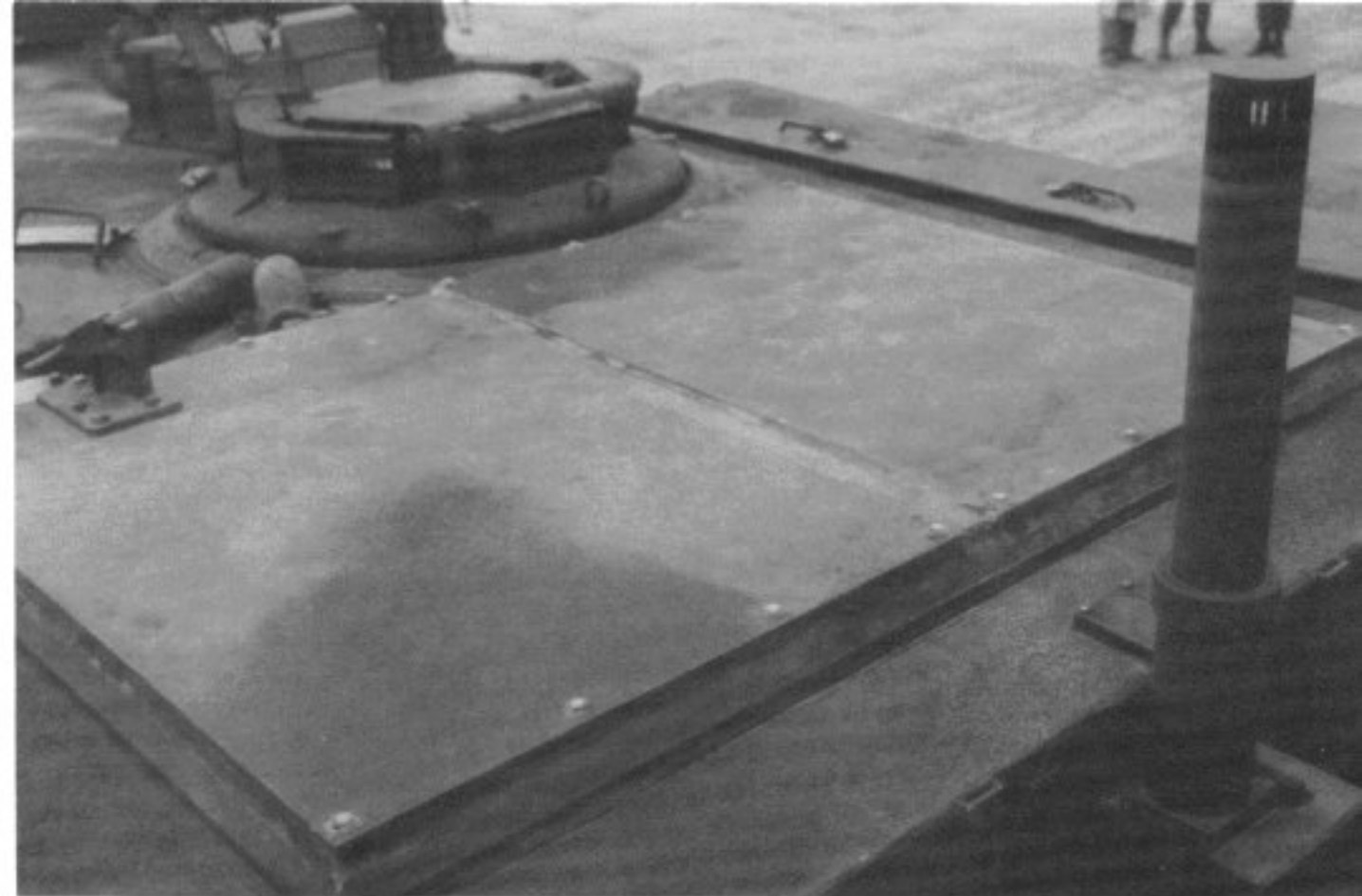
Production M1A1s feature the final blast panel configuration which consists of two equal sized turret blast panels in place of the earlier three panel configuration used on the M1. The wind sensor post has also been changed and now has a slimmer shape. (Jerchel)
