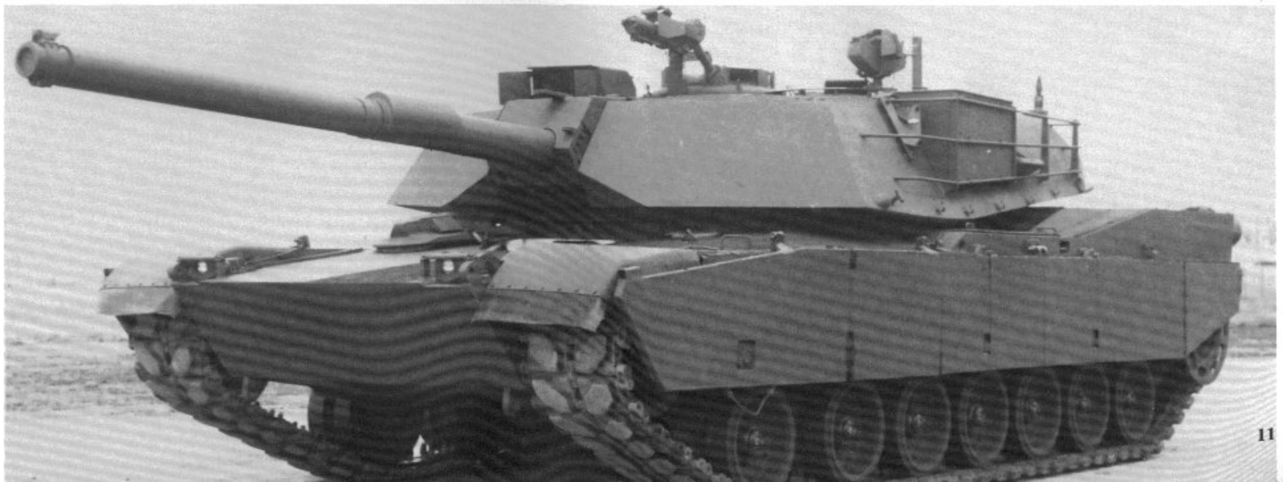
(Below) The M1 has a low sleek look compared to other US tanks such as the M48 and M60. The main external difference between production M1s and the trials vehicles was in the turret which was extended rearward by an eight inch plate at the rear of the turret. (Wagner)
