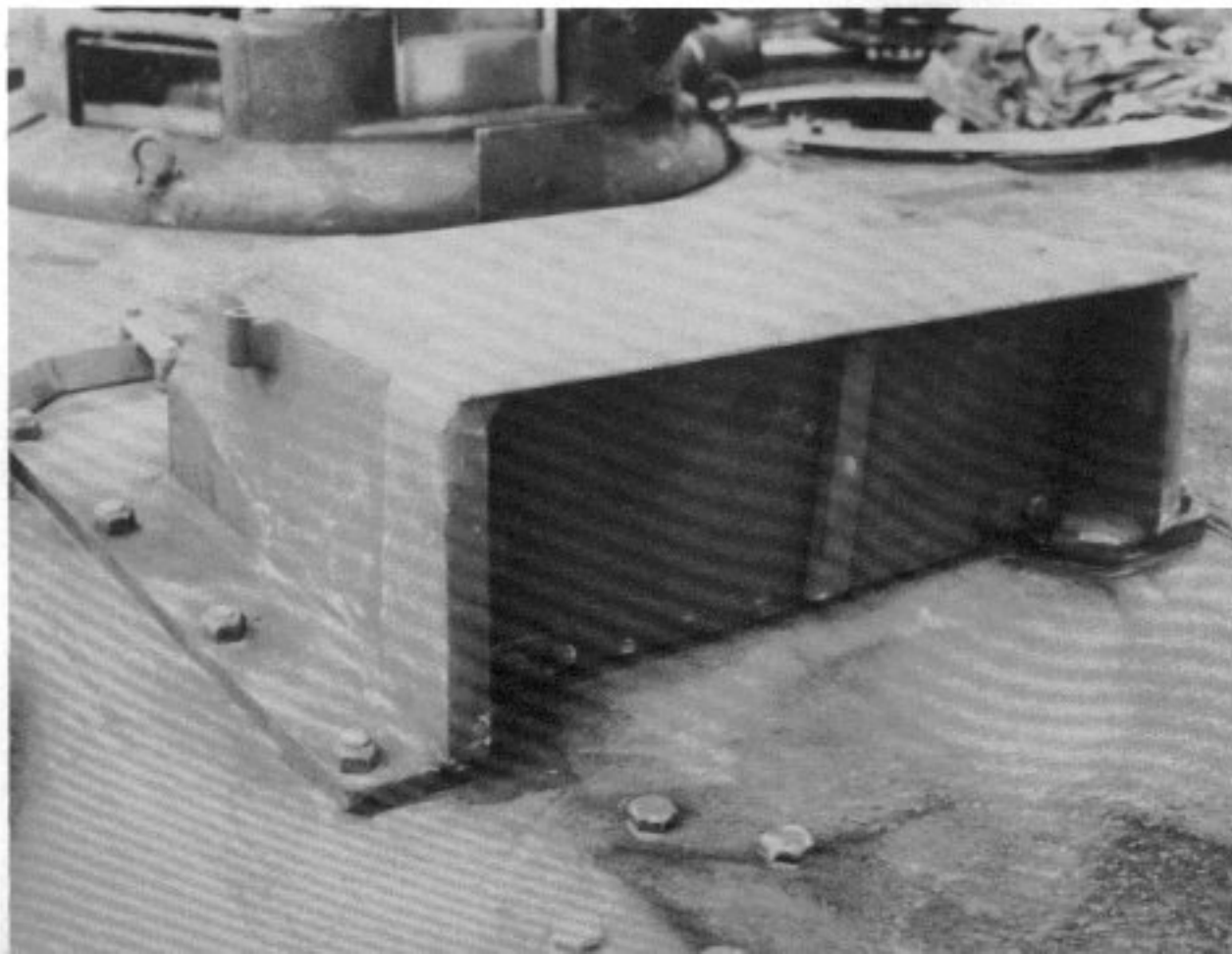
The gunners sight aperture on the M1A1 has been modified to handle upgraded optics. The armored doors on the front of the sight are now recessed and protected by a heavy metal lip. The doors swing outward when the sight is in use. (Sewell)
