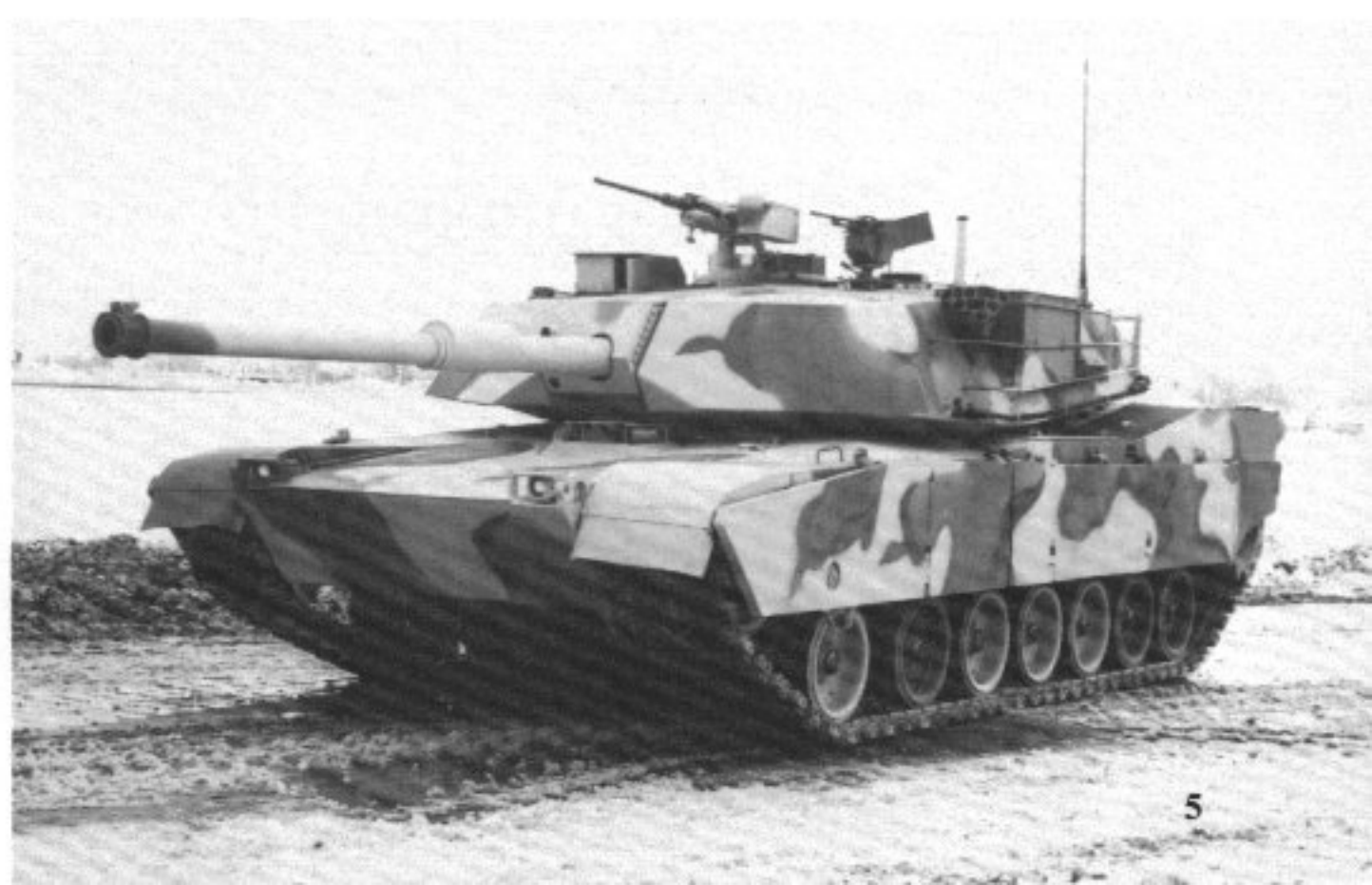
One of the XM1 pilot vehicles, painted in a three tone camouflage scheme, rests outside the Detroit Army Tank Plant during 1978. Extensive tests with these vehicles showed that the XM1 was a robust, reliable vehicle. The main problem areas encountered were with the turbine air filters, transmission, and fuel supply. (Wagner)
