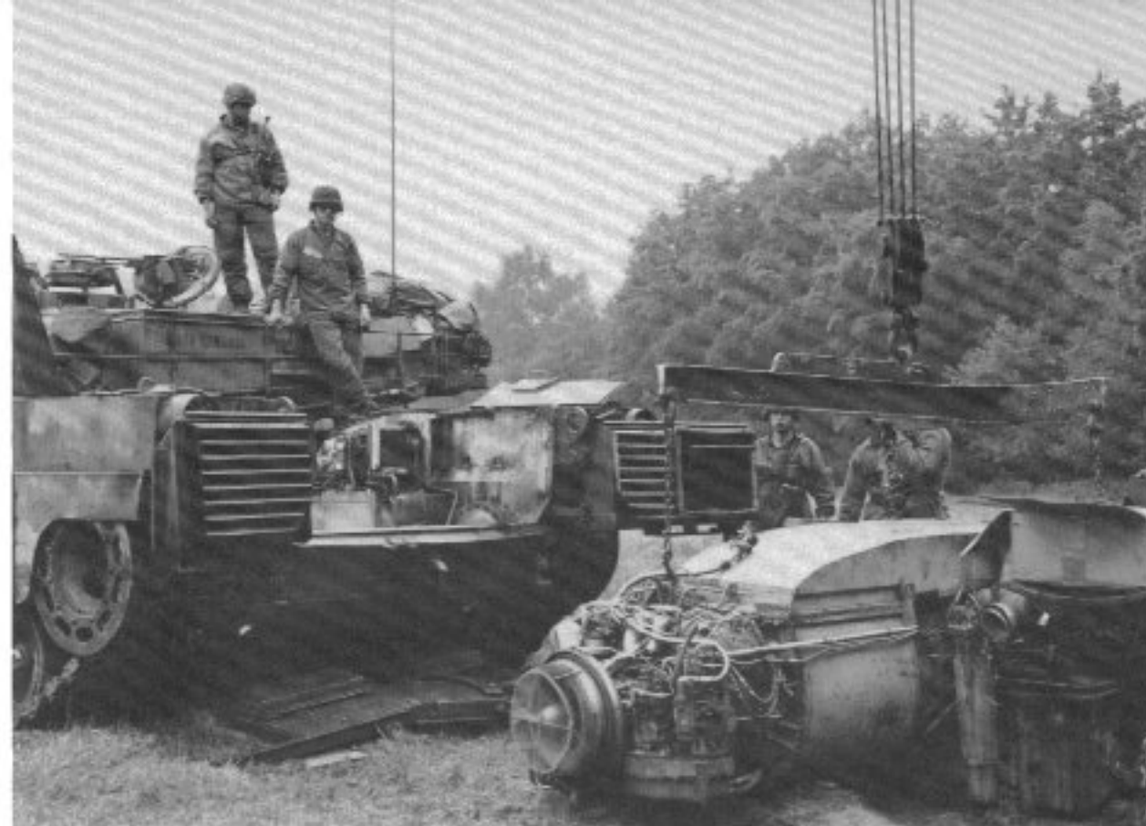
Changing a power pack on the Abrams can be done in the field in about an hour, enabling the tank to quickly return to action. This is a dramatic improvement compared to the four hours needed to replace an M60 engine. (Jerchel)
