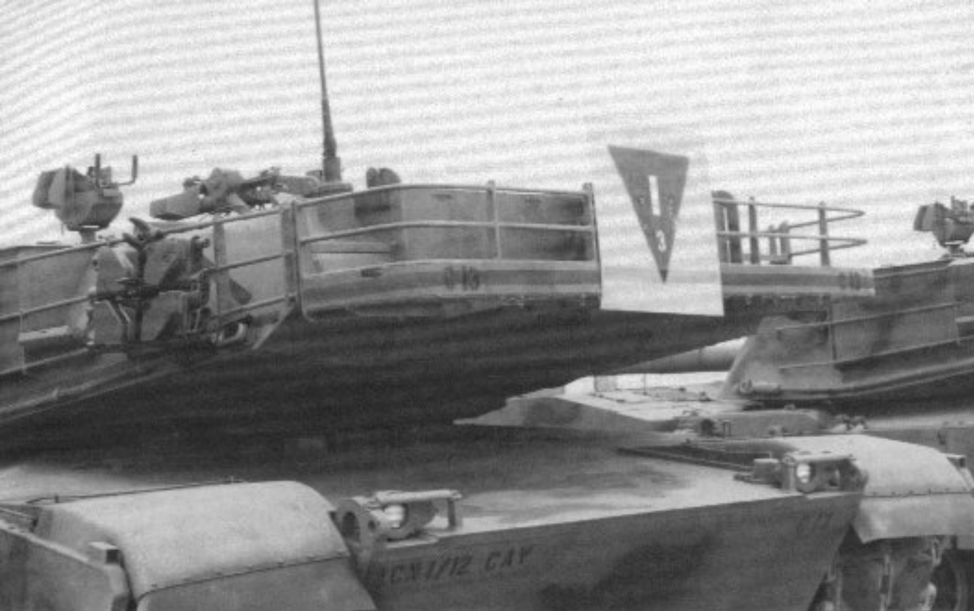
The rear stowage rack is hinged to swing up and out of the way to allow the crew access to the engine deck. The Black strip along the metal lip is a velcro strip for attaching Multiple Integrated Laser Engagement System (MILES) laser training gear to the tank. (Mesko)
