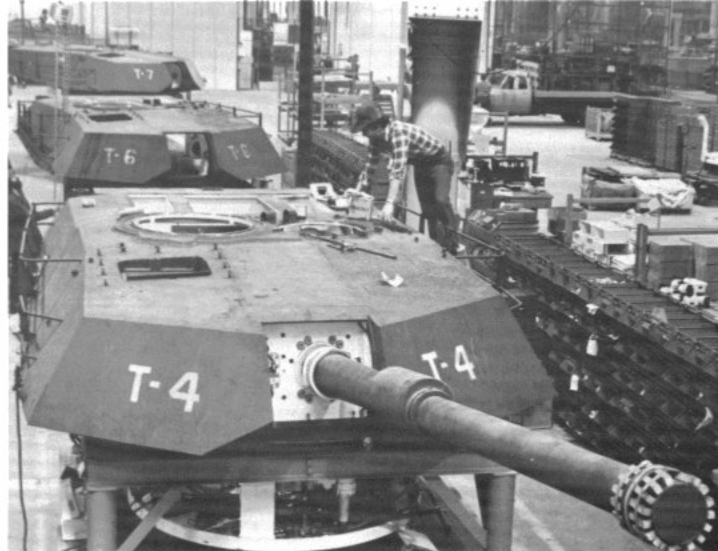
(Above) A nearly complete turret, fitted with the 105mm gun and turret basket, moves down the assembly line. The screws sticking up in front of the commander's station mark where the cover for the gunner's sight will be located and bolted down. (Wagner)
