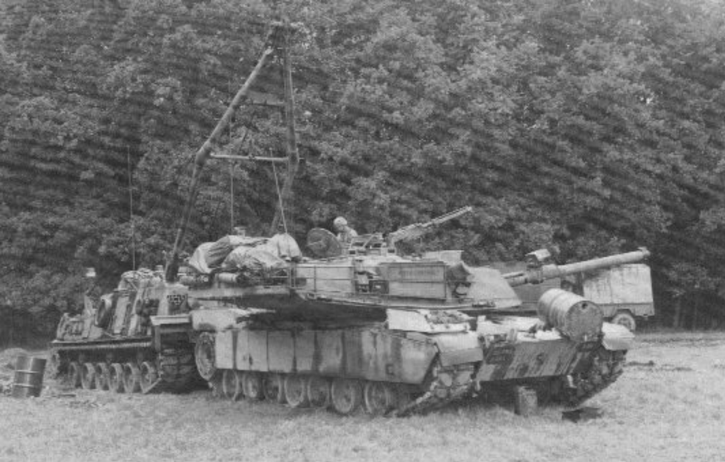
The Abrams has proven relatively trouble free in the field. When problems have occurred they have been handled quickly by repair crews. The crew of this M88 recovery vehicle helps pull the engine pack on Birth Control , an M1 from the 2nd Armored Division during exercise Certain Strike . (Jerchel)
