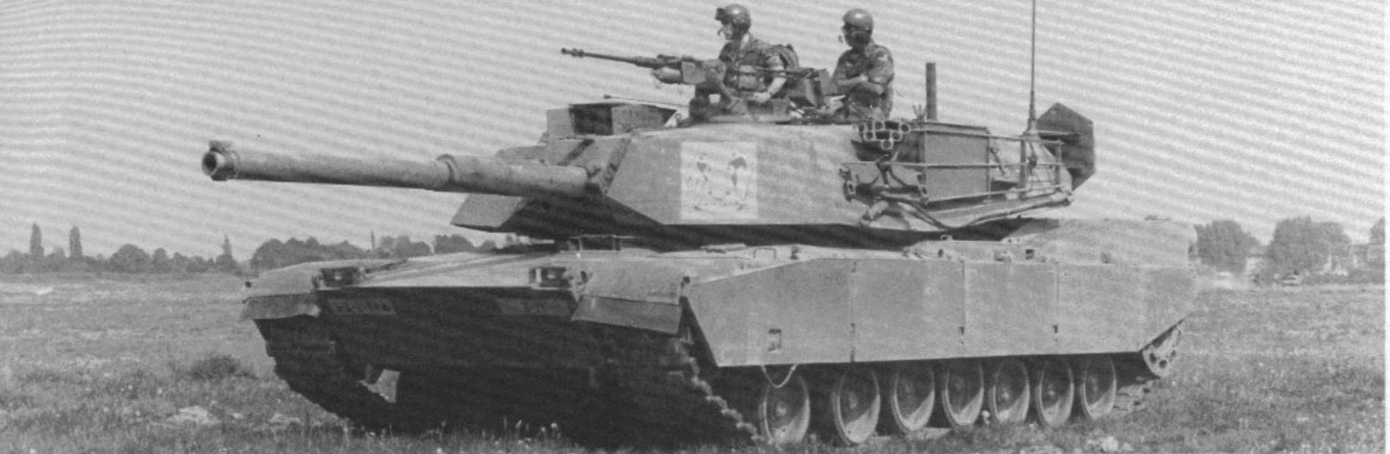
(Below) M1s moving cross country at high speeds can create a large dust cloud. The M1 can also create a deliberate smoke screen by using its grenade launchers and engine smoke generator when under enemy fire. (U.S. Army)
