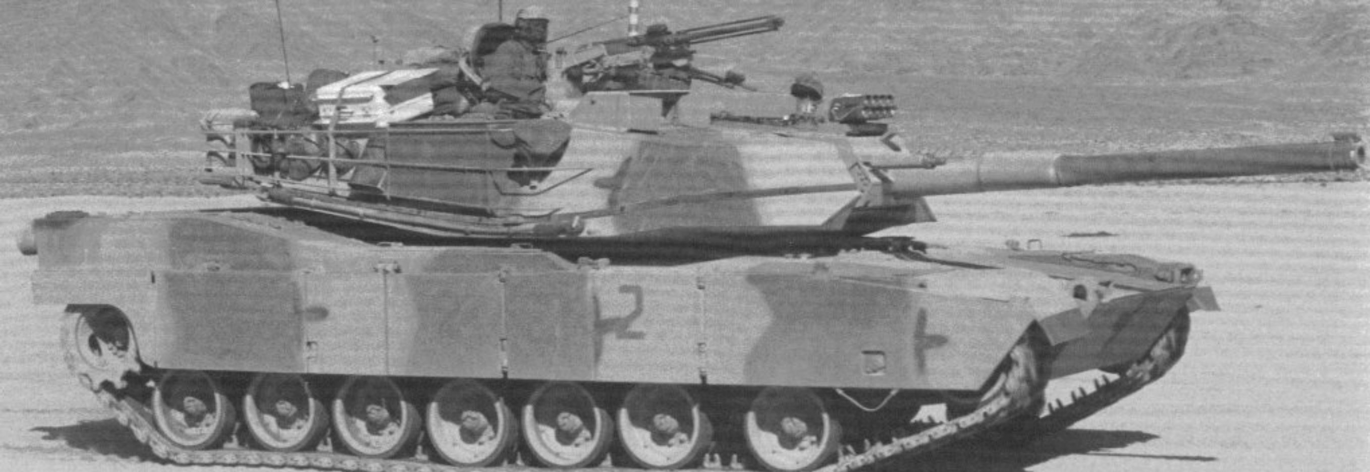
(Above) Eventually a number of M1s were permanently assigned to the NTC for use by units deployed there for training. M1s at the NTC were painted in a desert camouflage scheme and had removable numbers on the armored side skirts made from Green tape. (Green)
