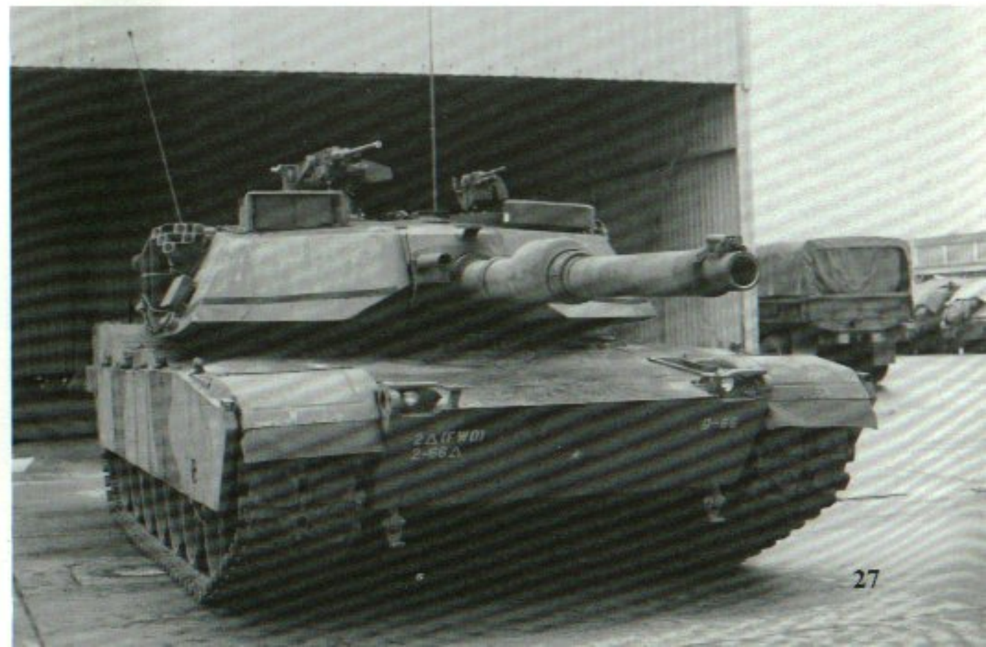
The headlight guards on the M1A1 differ from the M1 being flatter and slanted slightly forward. These revised guards also have a slight dip on the top and have only one attachment bolt. (Jerchel)
