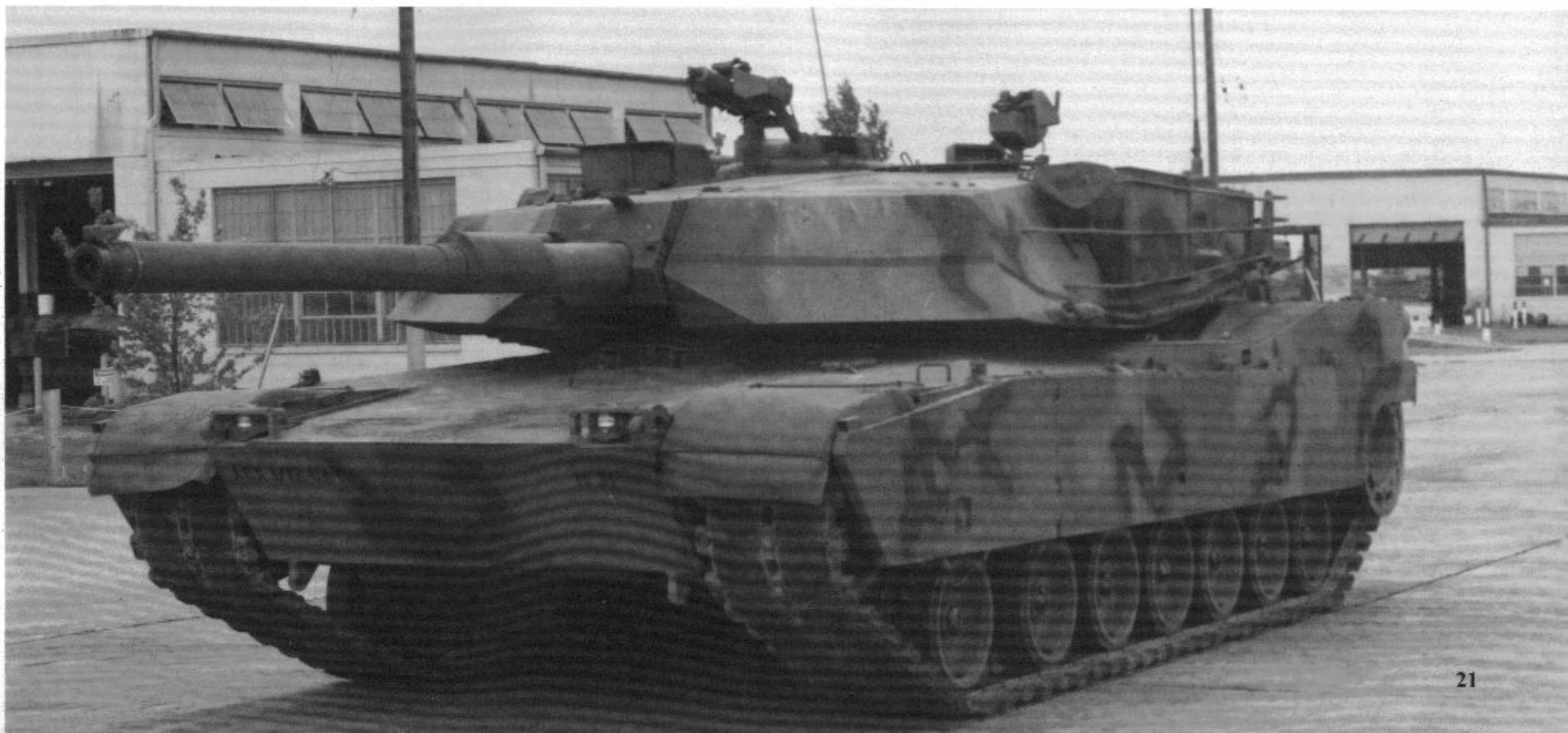
The distance between the gun bore evacuator and mantlet is shorter on the IP M1 because of the addition of extra armor on the turret face, however, overall barrel length is actually unchanged. (Mesko)
