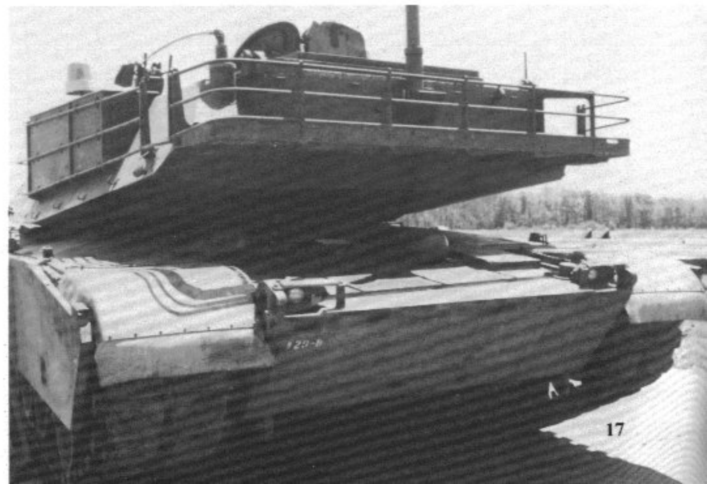
The new armor configuration under consideration would also add more protection to the hull. External armor plates were welded to the front of the hull to simulate the additional weight of the proposed change. (Green)
