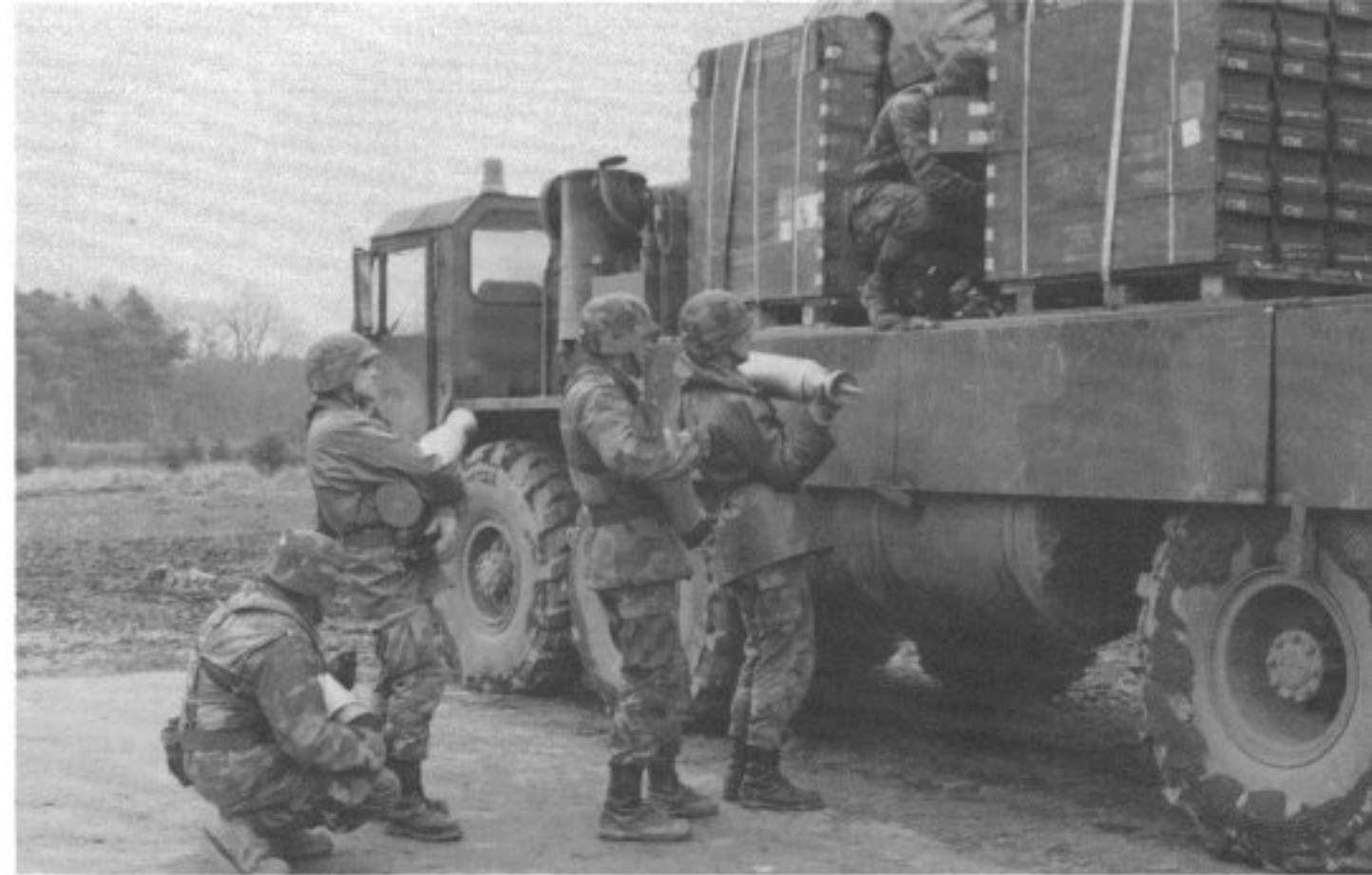
Tankers unload practice rounds from a M977 HEMTT. Each pallet of ammunition has thirty rounds on it and the M977 can carry a total of eight pallets (240 rounds), enough to supply six M1s with a basic combat ammunition load. (Jerchel)
