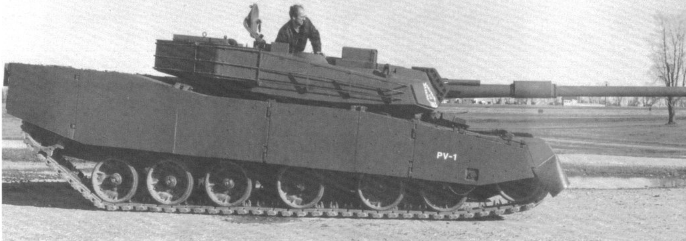
(Above) The XK-1 features a combined torsion bar/hydro-pneumatic suspension which allows the tank to "kneel" for additional depression of the main gun. The system also gives the vehicle a smoother ride over rough terrain. The first two and last bogie wheels are pneumatic while the middle wheels are attached to a torsion bar. (Green)
