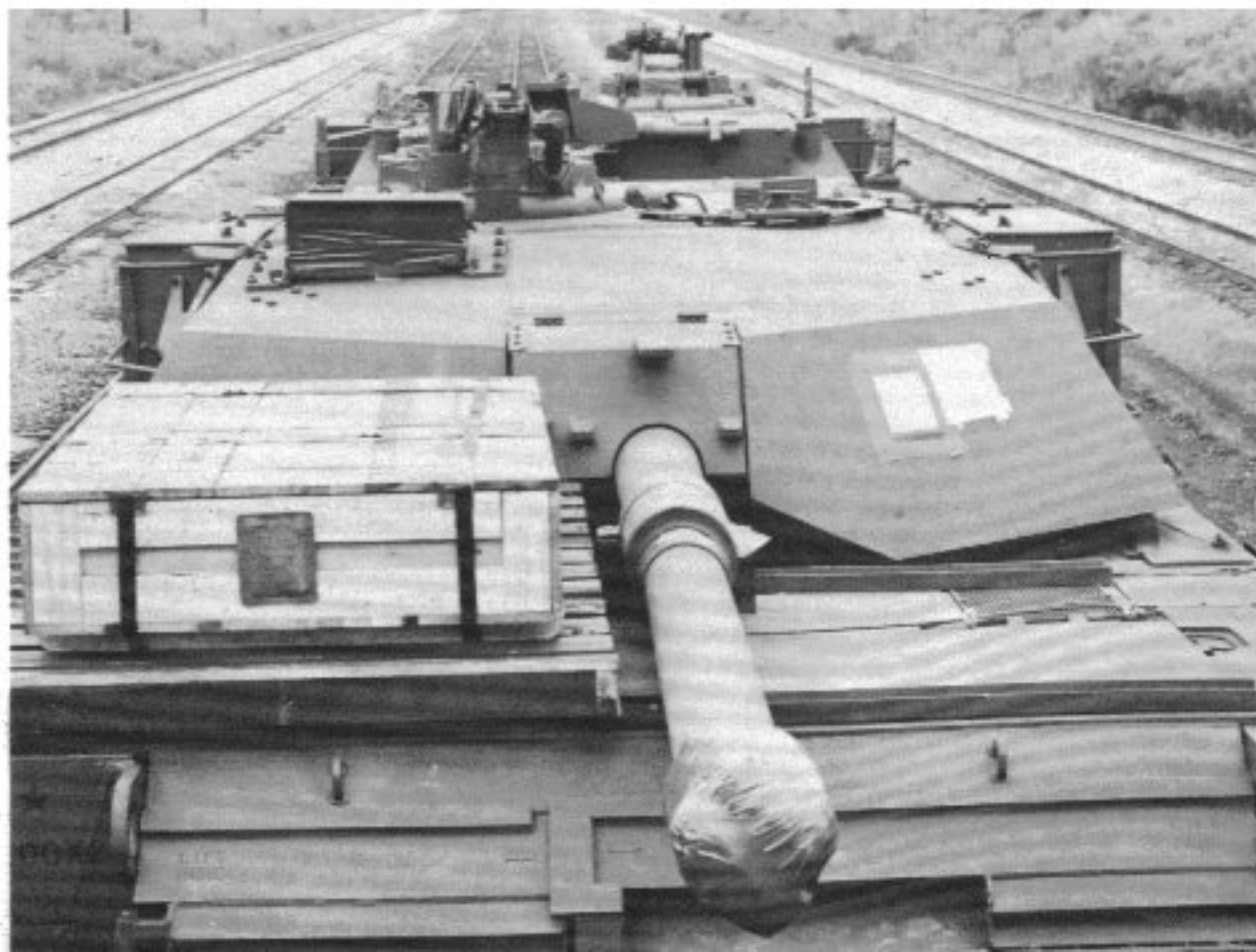
Additional equipment for the M1 is stored in the wooden box secured to the rear decking. Besides covering the gun barrel opening, the protective tape also covers the muzzle reference system to protect it from damage. (Mesko)
