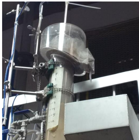
3 inch column flotation Pilot
